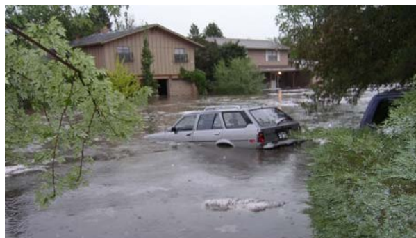
Photo 4. Overflow area at sump was blocked with landscaping and fencing, resulting in flooding.
