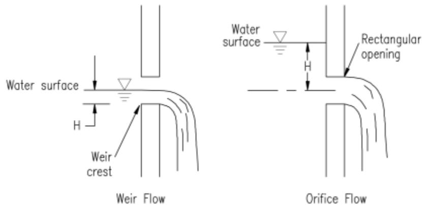
**Figure 3-10: Weir and Orifice Flow**
